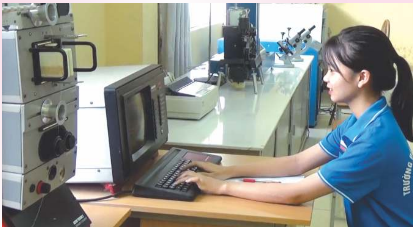
Fiber and textile students are practising testing yarn quality on Uster Tester 3.
